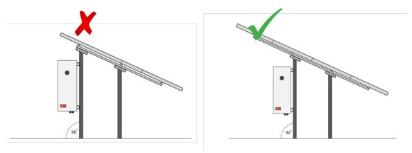
• DC Combiner shall be mounted in a way that guarantees that is not in the path of rainwater flowing off/between the module frames.
